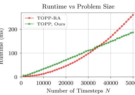
QOPP is as-fast or faster than TOPP (C++) Runtime is O(n) w.r.t. trajectory length
