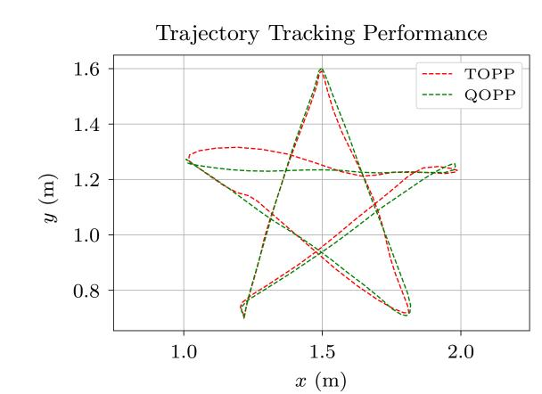
As a result, executing on a real robot, TOPP has poor tracking performance (QOPP is still good).
