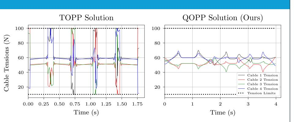
TOPP constantly hits control limits. Meanwhile, QOPP allows us to trade-off speed for control margin.
