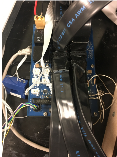
Figure 4: sbRIO-9627 module with 3 current sense inputs, 3 hall sensor inputs, and 96 MMSPC logic outputs
