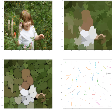
Figure 16. Example 7 - A small girl on the grass play. Output image from Clip, segmented image (68 segments), output “painting”, and robot trajectories.
