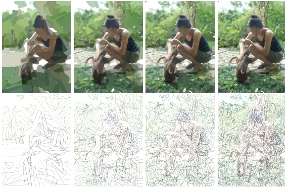
Figure 19. Rendered paintings of trajectories optimized by diffvg using (left-to-right) 64, 256, 512, and 1024 strokes. On the top row are the rendered paintings and on the bottom row are the robot trajectories with colors.
