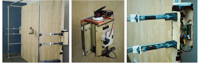
Fig. 6. Our cable robot (left) includes an end effector that carries the spray paint and actuator electronics (center) and 4 winch assemblies, each consisting of a shared motor controller, motor, and helical winch (right, x2).
