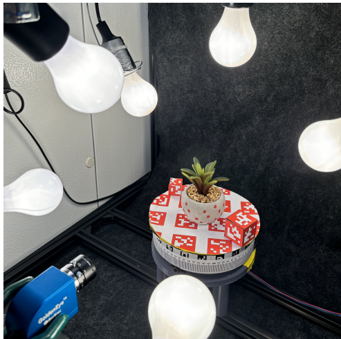
Figure 4. The BaySpec GoldenEye camera is held with a laboratory clamp and the sample of interest (here, an Anacamperos plastic plant) is placed on a turntable under tungsten halogen lighting. The camera is roughly 20 centimeters away from the scene thanks to its wide field of view.
