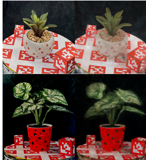
Figure 8. A demonstration of image sensor simulation ( Anacamperos top, Caladium bottom). Left: A photo taken with a smartphone (a crop from Fig. 4). Right: The simulated photo computed from the HS-NeRF.
