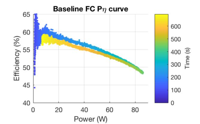
We first optimized pressure. Typically, higher pressures improve efficiency, as shown by the Nernst equation. However, in our case, the pressure differential across the membrane increased H<sub>2</sub> crossover, reducing efficiency.
