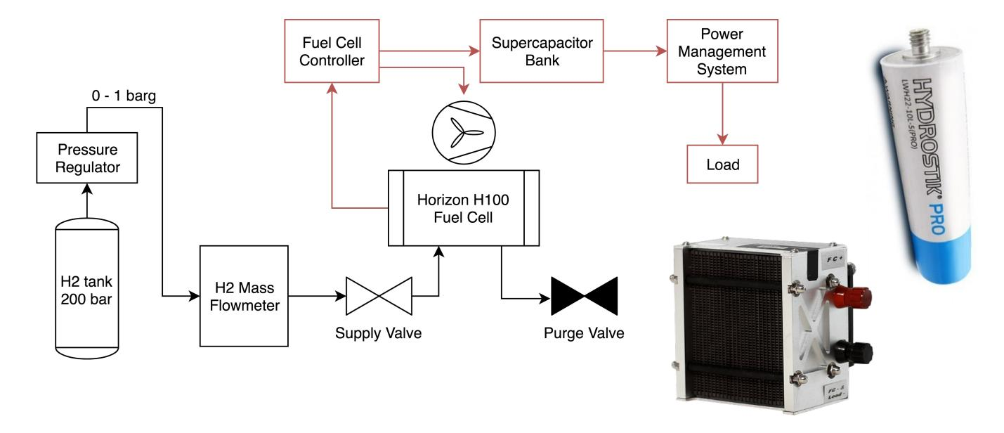
For the actual vehicle, Hydrostik PROs were used, which are metal hydride storage cylinders for hydrogen. These store hydrogen in chemical bonds, so they are compact and lightweight. A Horizon 100W FC was used for this study.
